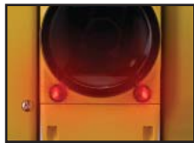
Layout Alignment Guide Lights Bright, focused LED guide lights assists in getting your rod man on line quickly.
